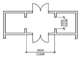
UDS Figure 4.2-23 Face of finish wall dimensioning.
