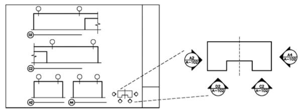
UDS Figure 4.3-2 Key plan used to identify the location of each elevation.
