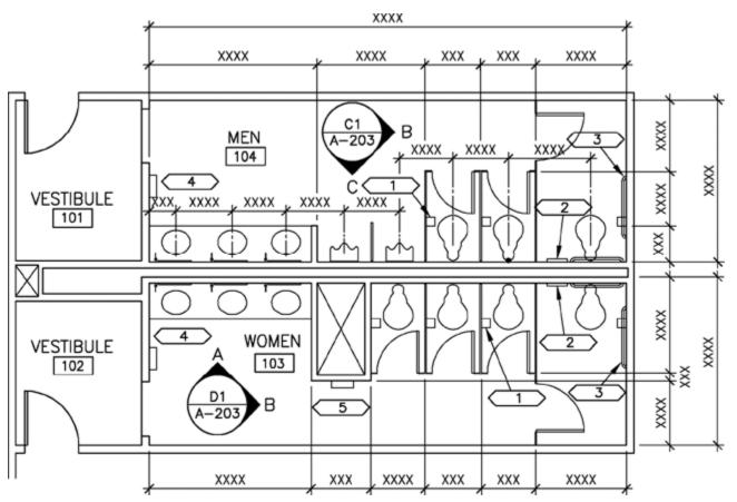
UDS Figure 4.3-10 Example of a toilet plan showing dimensioning, accessory identification, and reference to elevation.
