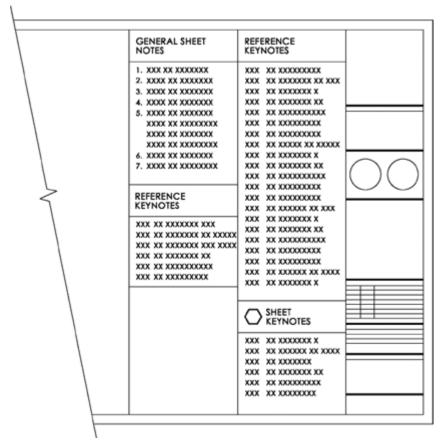
UDS Figure 7.3-11 Additional note blocks-an example using full and partial note columns.
