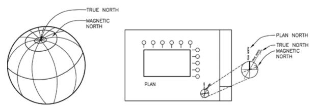
UDS Figure 4.2-2 Diagrammatic illustration of north arrow.
