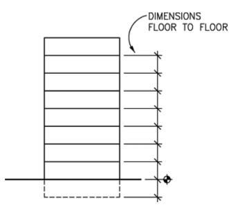
UDS Figure 4.2-25 Vertical section or elevation dimensioning.
