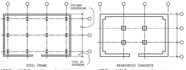
UDS Figure 04.19 Structural systems dimensioning.
