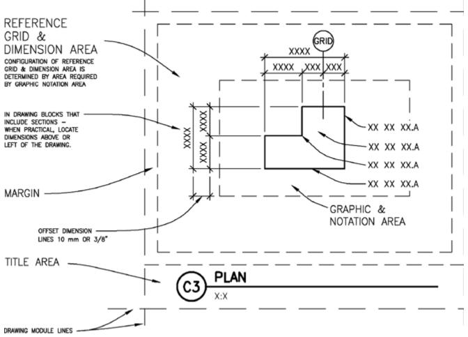
UDS Figure 4.2-26 Typical drawing block format.
