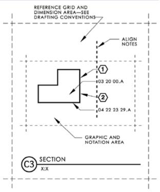
UDS Figure 7.4-1 Typical UDS drawing block format.
