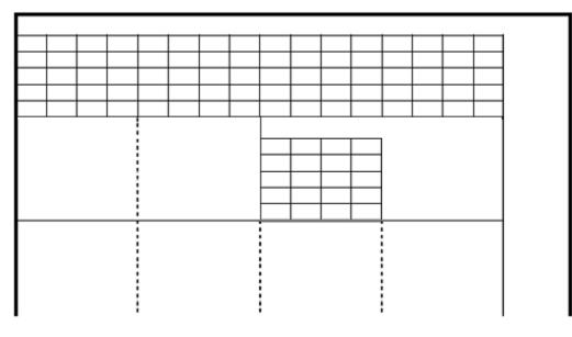
UDS Figure 3.5-1 Fitting a schedule into a drawing module.
