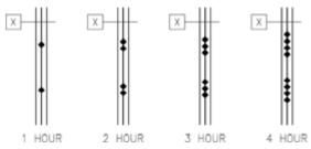
UDS Figure 4.3-24 Representation of fire-rated partitions on the floor plan.
