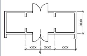
UDS Figure 4.2-22 Centerline of wall dimensioning.
