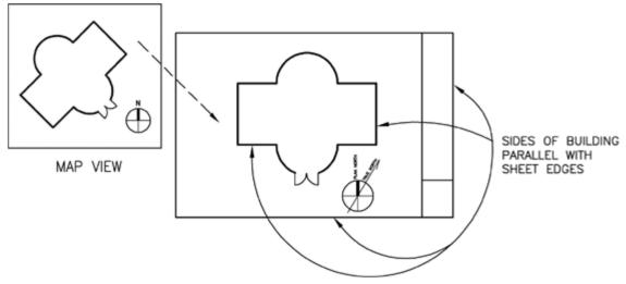
UDS Figure 4.2-1 Sheet layout orientation.
