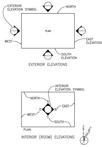
UDS Figure 4.3-5 Naming exterior and interior elevations.
