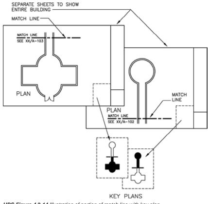
UDS Figure 4.2-14 Illustration of portion of match line with key plan.
