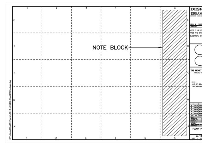
**UDS Figure 2.3-3.** If the sheet does not have a note block locate the key plan block in the lowest module next to the title block. Refer to <u>UDS Figure 4.2-14</u> in the *Drafting Conventions, UDS section 4.2*.
