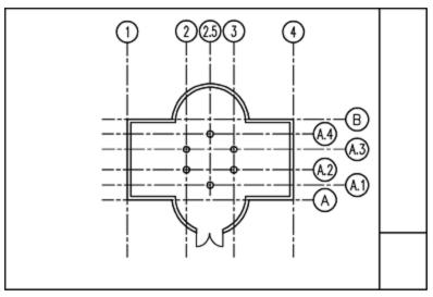
UDS Figure 4.2-5 Illustration of column grid line.
