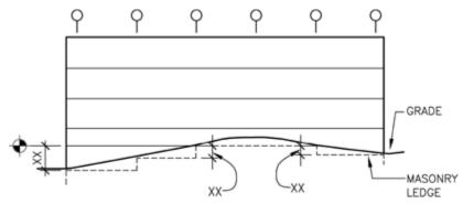
UDS Figure 4.3-4 Elevation at grade.
