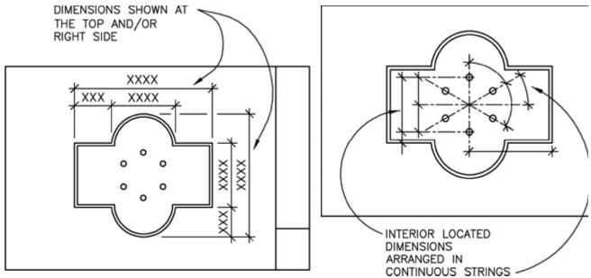
UDS Figure 4.2-15 Dimensioned floor plan, exterior dimensions.
