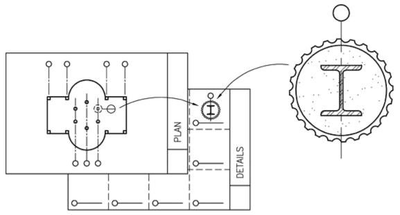
UDS Figure 4.2-4 Plan detail having the same orientation as the floor plan.
