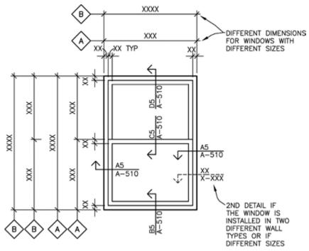
UDS Figure 4.3-21 Double-hung window type with dimensions representing two window sizes.
