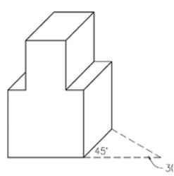
**UDS Figure 4.3-25** Axonometric isometric drawing.
