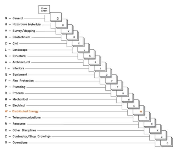
UDS Figure 1.2-1 Illustration of a typical drawing set.
