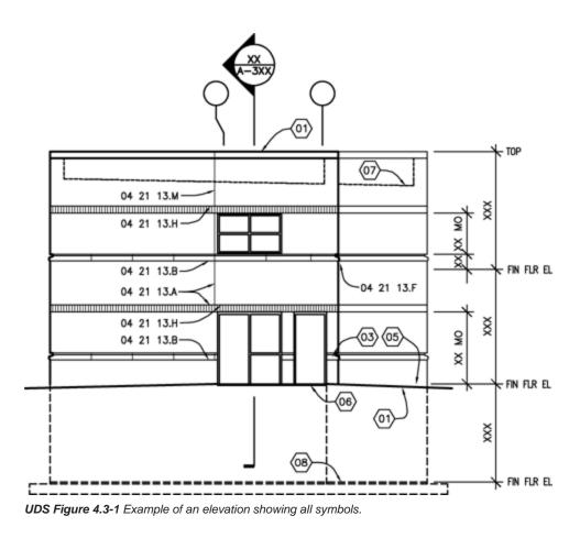
If a Key plan is used on the plan sheets, it should also be placed on the elevation sheets with elevation symbols indicating the location of each elevation shown on the sheet. Refer to **UDS Figure 4.3-2**. Match lines should be set at the same locations as the plans. Grid lines should be placed only at corners and where changes in planes occur.
