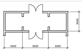
UDS Figure 4.2-21 Face of stud, concrete or masonry wall dimensioning.
